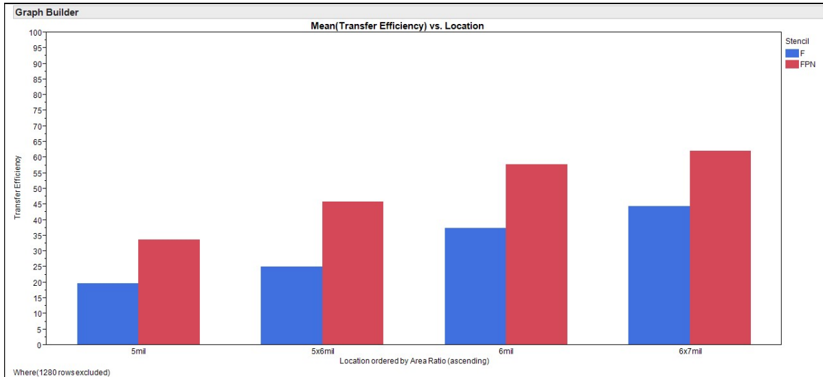
Figure 15 – 03015 Metric Stencils Mean TE% by Aperture Size, 3 mil Thick Uncoated (F) (Blue) and Nano-coated (FPN) (Red) Stencils, Type 5 Solder Paste
